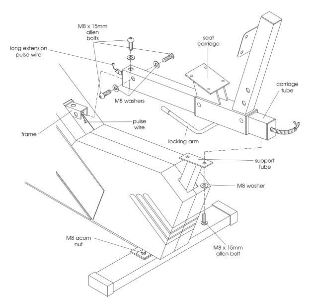
Figure 3 - Assemble Seat Carriage
